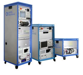
GÖPEL electronic has specialised in the area of networking test systems for automotive control devices for many years and is the leading provider of network testers. This has resulted in the creation of a modular and OEM-independent system, which can be used across buses. In the foreground there are CAN, CAN-FD, LIN and FlexRay as well as future bus architectures such as Automotive Ethernet (BroadR Reach).
